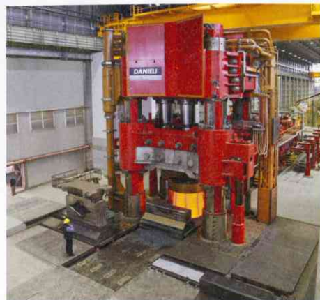
Cover photo: 110-MN open-die forging press with four prestressed columns and a welded steel structure, at Fomas Group, Italy
