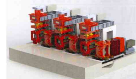
Roughing mill in H/V configuration
